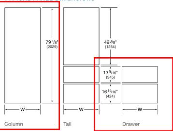
Typical panel dimensions are based on an 84" (2134) finished height for column and tall models and 341/2" (876) for drawer models, with a 4" (102) toe kick and 1/8" (3) reveals. Panel dimensions must be adjusted accordingly for all other installations. Refer to the illustration for panel heights and the chart below for panel widths.
