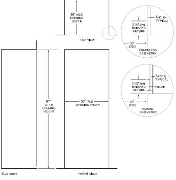
NOTE: 3'/2" (89) finished returns will be visible and should be finished to match cabinetry
