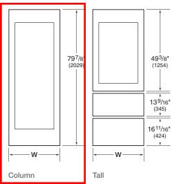
Typical panel dimensions are based on an 84" (2134) finished height, 4" (102) toe kick and 1/8" (3) reveals. Panel dimensions must be adjusted accordingly for all other installations. Refer to the illustration for panel heights and the chart below for panel widths.
