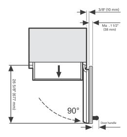
When installing hinge side next to an appliance or object that is within range of the door panel, limit the door opening angle to 90°. This is done by installing the banking pin as illustrated. Insert the banking pin through the holes and drive in with a hammer.
