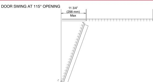
**NOTE**: Additional space needed depending on thickness of front panels and handle used
