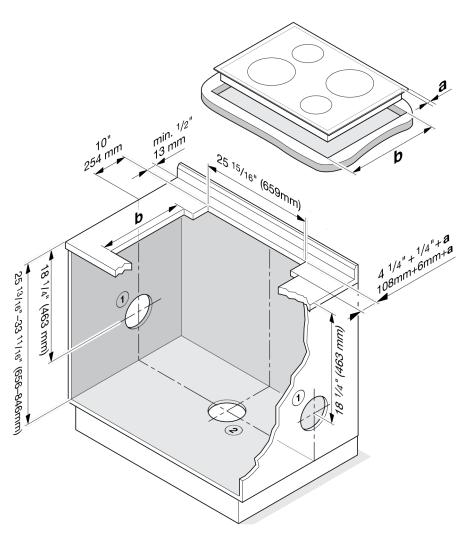
Exhaust or recirculation mode with DAG 600 blower installed at the front of the downdraft. Exhaust ducting ( $\varnothing$  6" (150 mm))
