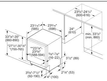
\* measured from the bottom edge of the countertop panel thickness recommended 3/4" (20 mm).
