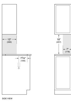
NOTE: Shaded area above countertop indicates minimum clearance to combustible surfaces, combustible materials cannot be located within this area.
